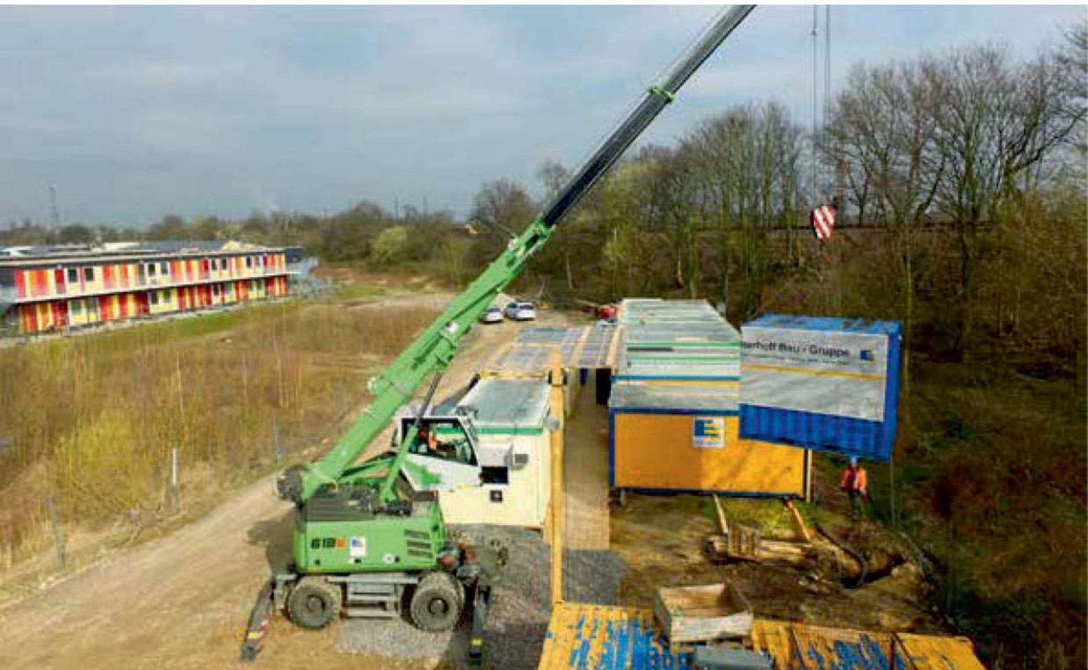
613 M - flexible 16 t construction site crane with overview due to elevating cab; Germany
